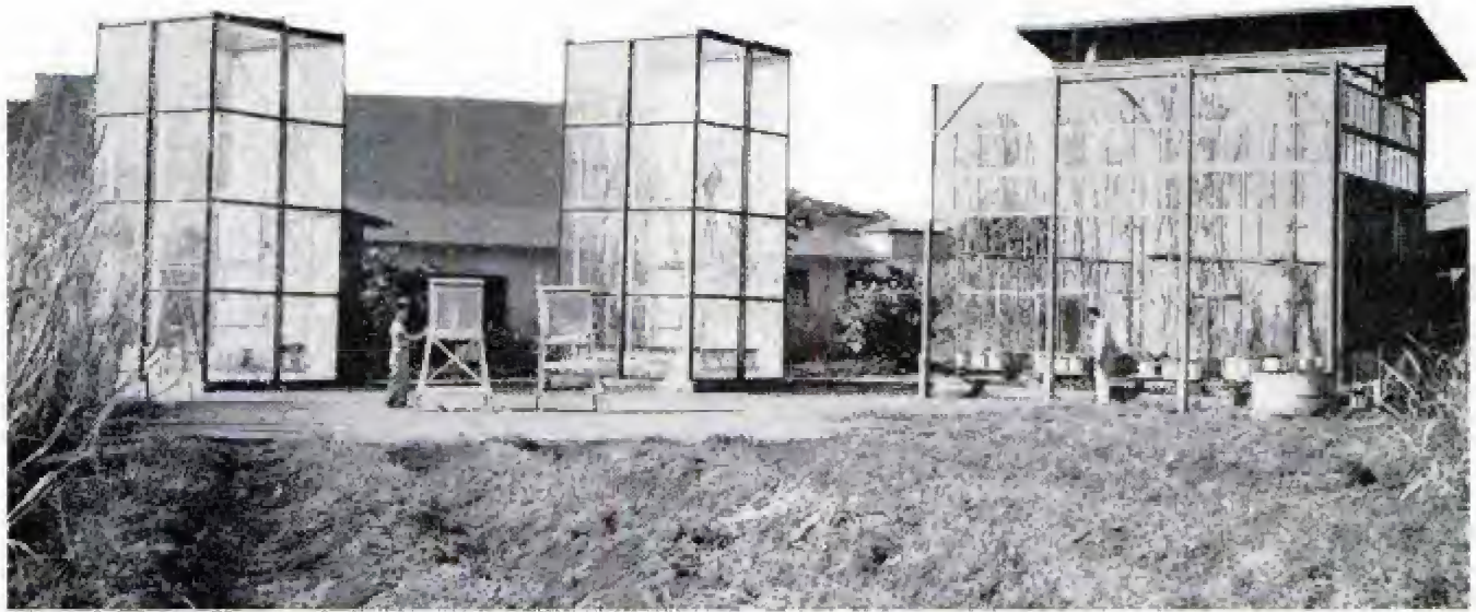
Sugar cane is raised in weather-controlled glass houses to determine the effect of temperature on its growth
